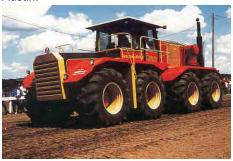
Big Roy was built by Versatile in 1977 at its plant in Winnipeg. The largest tractor ever built the Versatile 1080 (Big Roy) was actually too heavy to use as its tires compacted the soil too much. They tried to alleviate this by tripling the number of wheels. The result was a tractor with 24 wheels that was nearly impossible to turn.
